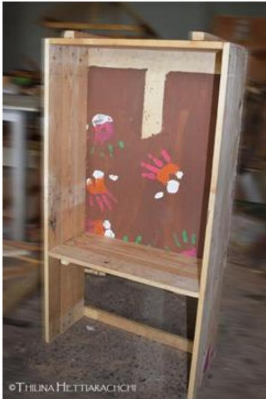
**Figure 3. make a frame/or wooden box first. The box should be a minimum of 20cm deep and open only from the front**
